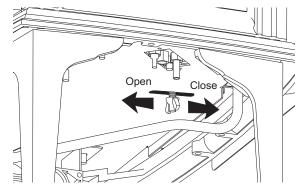
Figure 25. Loosen the wingnut to adjust the air shutter.
